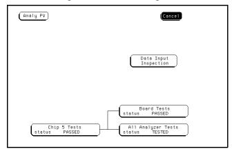
**6** Select Run, then select Single. The test runs one time, then the screen shows the results. When the test is finished, select Done.
